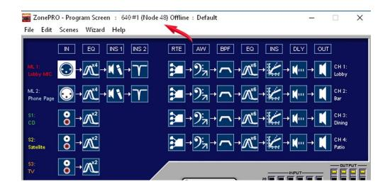
B. Click the top router (RTE), then press [Ctrl]+[Shift]+[o]. The Object ID information window will open. Enter Address b0 (Index) into the "Address Object ID (b0)" field. Then enter Address b1 (Row) into the "Address Object ID (b1)" field.
